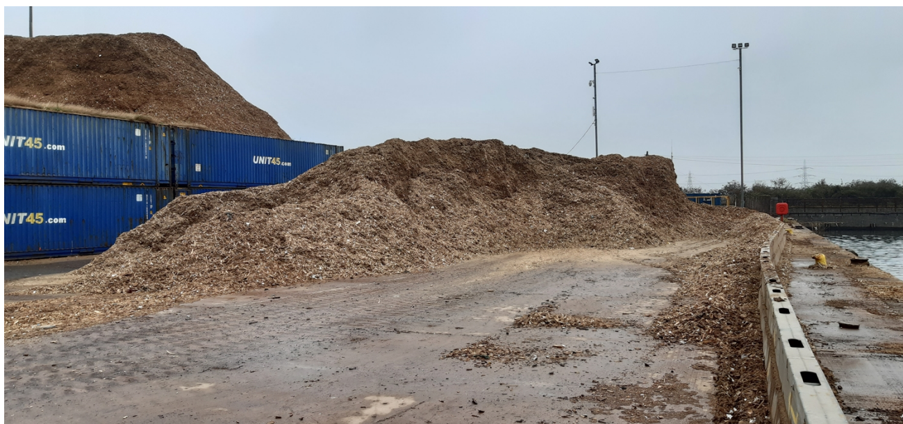
Photo 2 - ABP Site with sufficient fire breaks in place
