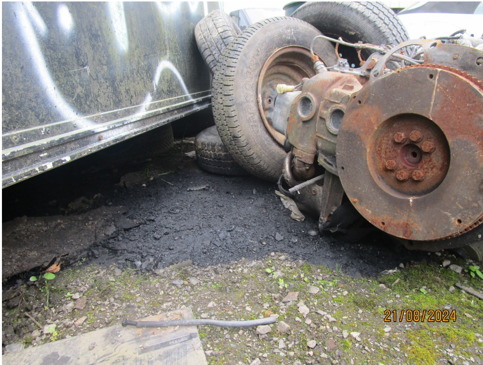
Figure 5. Oil leaked to ground from vehicle parts
