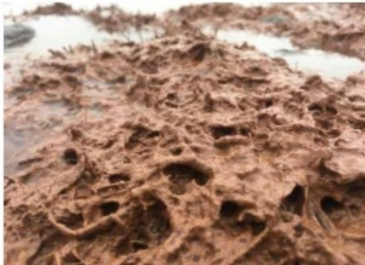
Close up FlocMat showing accretion of silt
