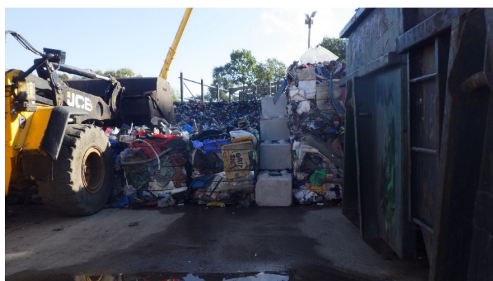
Waste stored higher than concrete fire walls
