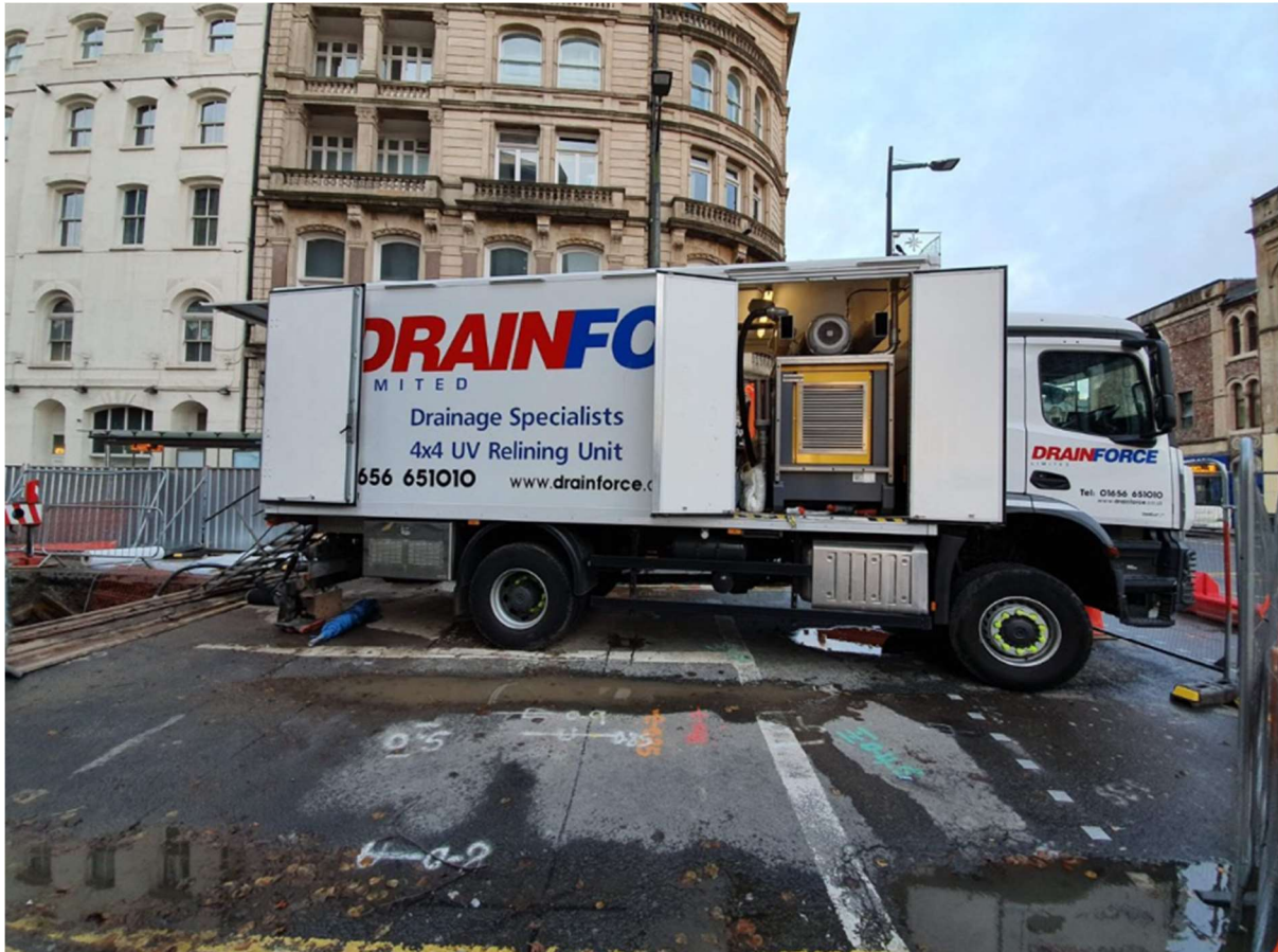
Fig 10 – Photo of DrainForce UV Rig.
