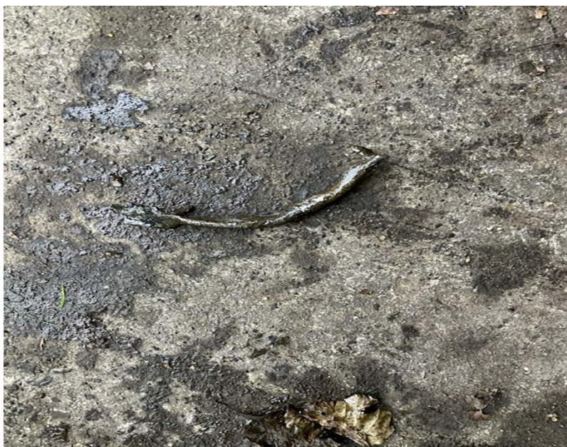
Third-party metal object which blocked one pump at Aberbanc SPS on 02 November 2024 (photograph courtesy of DCWW)
