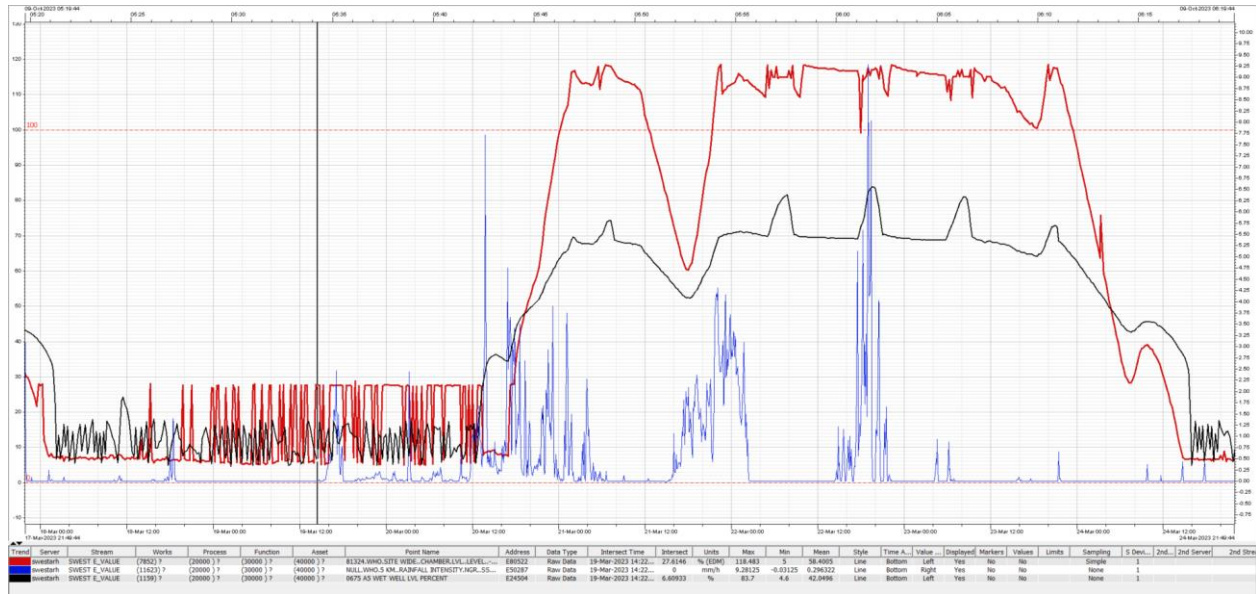
Figure 3 - Red displays levels at CSO. Dotted red line indicates spill level. Blue displays rainfall. Black displays SPS wet well levels. Data indicates direct link to rainfall events, and spills occurring only when SPS wet well levels are high.
