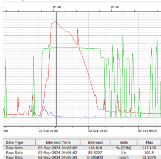
Figure 5 - Red displays levels at CSO. Dotted red line indicates spill level. Blue displays rainfall. Green displays SPS Pass forward flow.
