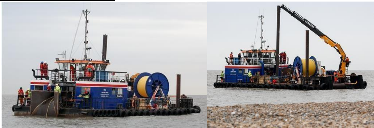
Figure 5: Multicat Vessel Equipped for Cable Installation
