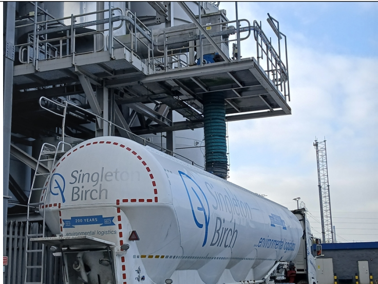
APC residue collection from silo
