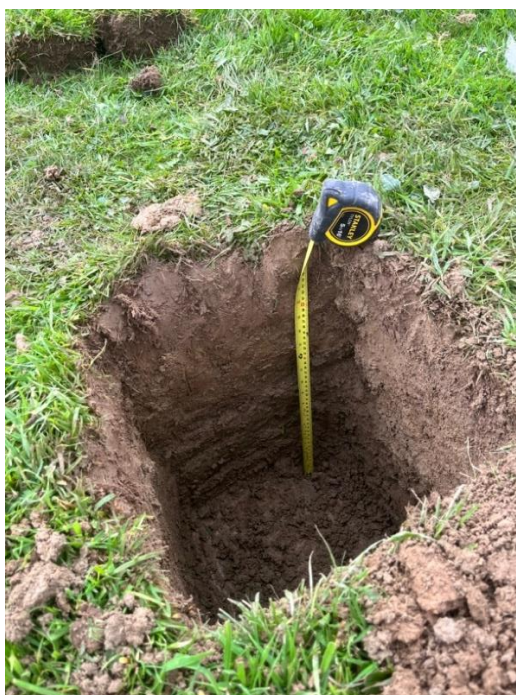
Figure A3 - Percolation test hole 1
