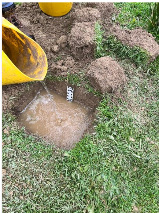
Figure A4 - Percolation test underway
