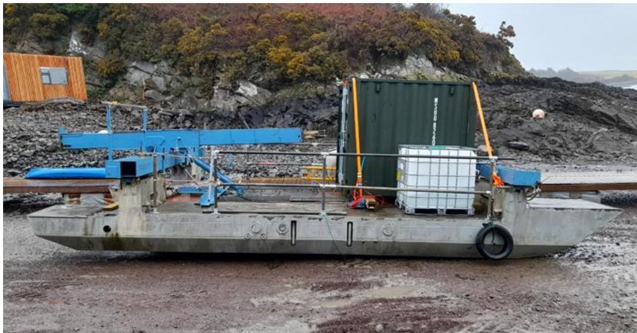
Figure 3 The 10 x 6m barge that the blade and arm will be attached to.
