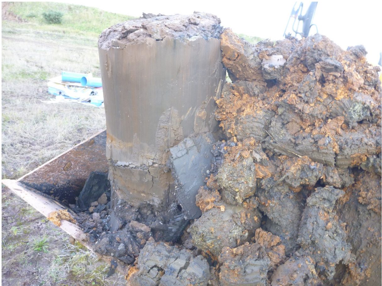
Photograph 2: Typical arisings from drilling in cell 0 and 1, the orange colour is the deposited filter cake.
