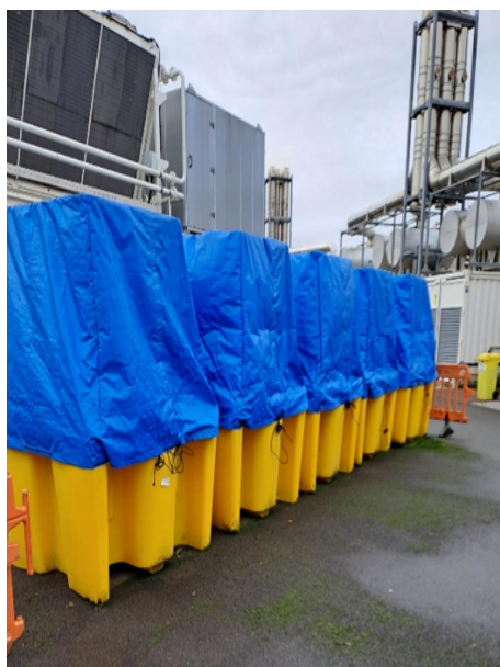
IBC Sub Pallet with Rain Guard
