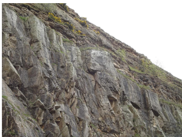
Plate 9: Close-up of Plate 8 showing incipient failure on joint sub-parallel to major problematic feature.
