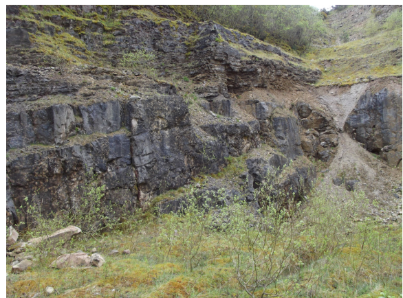
Plate 11: Ravelling failure at face corner
