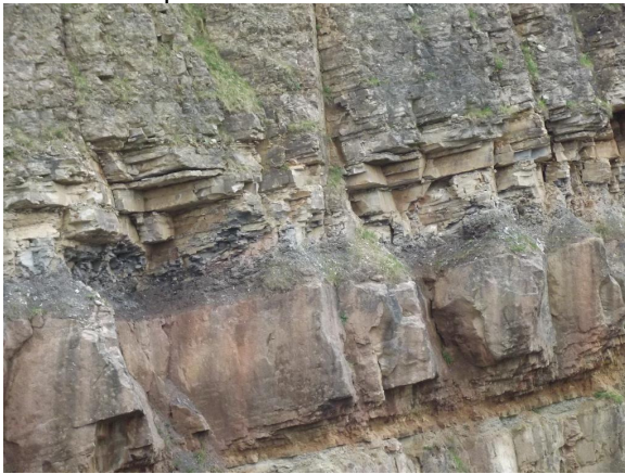
Plate 12: Close-up of preferential weathering along soft shaley bands
