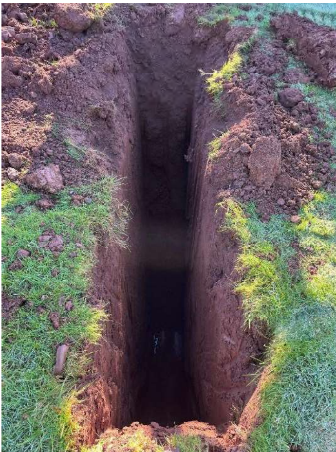
Figure 2-10 TP03 water seepage
