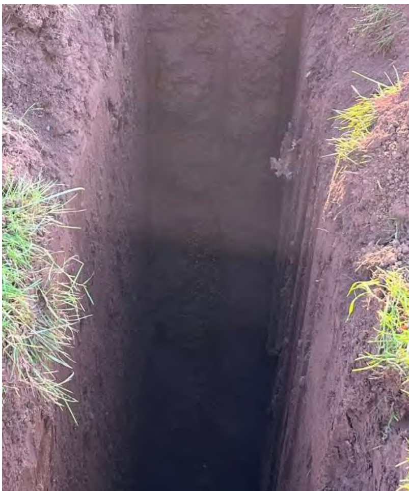
Figure 2-11 TP03 close up water seepage 0.8mBGL
