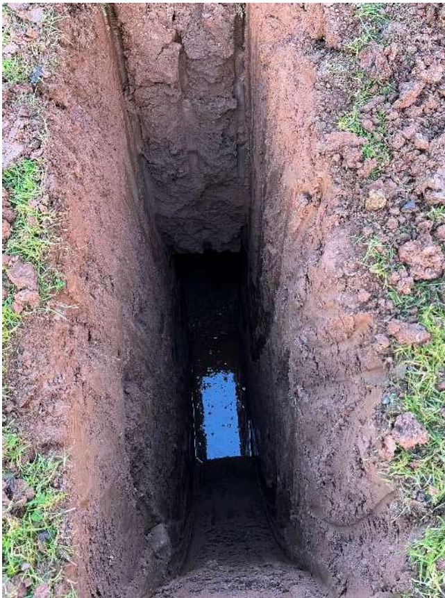
Figure 2-4 TP01 end of water seepage
