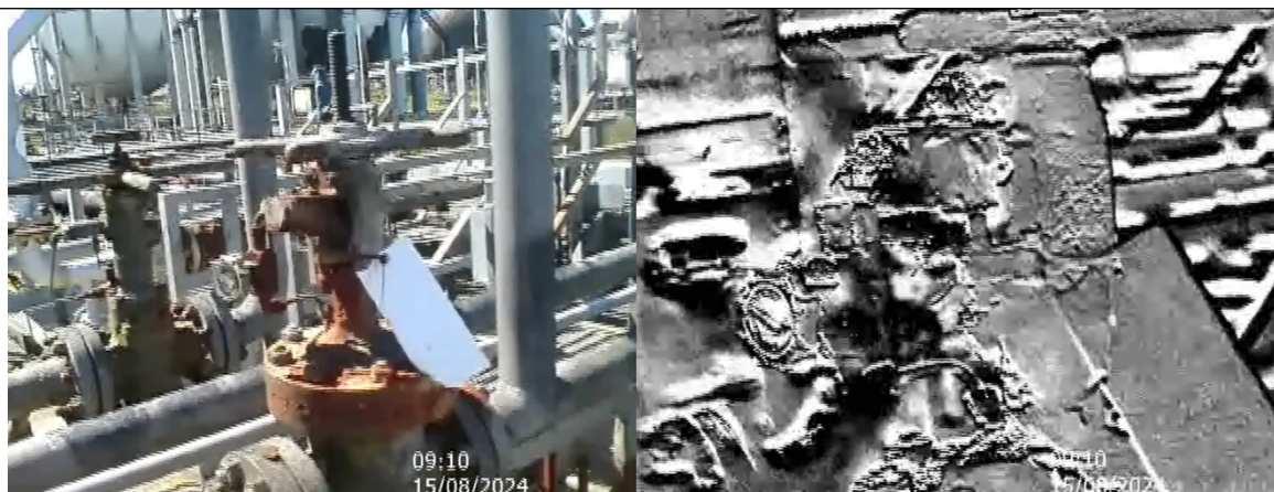
Optical Gas Imaging camera recording, right image showing infrared mode capturing gas leaking from valve (black haze)
