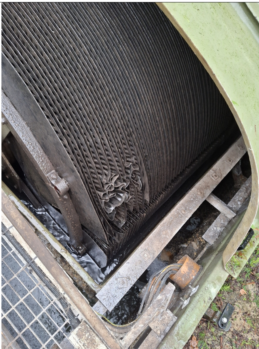
Figure 2 RBC appeared to be in good working order at the time of inspection
