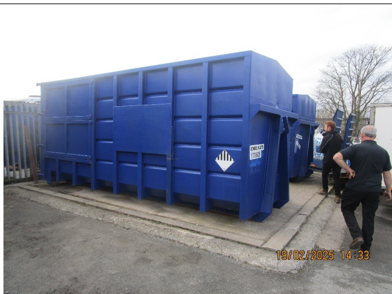
Figure 1. Both skips stored on an impermeable surface connected to sealed drainage
