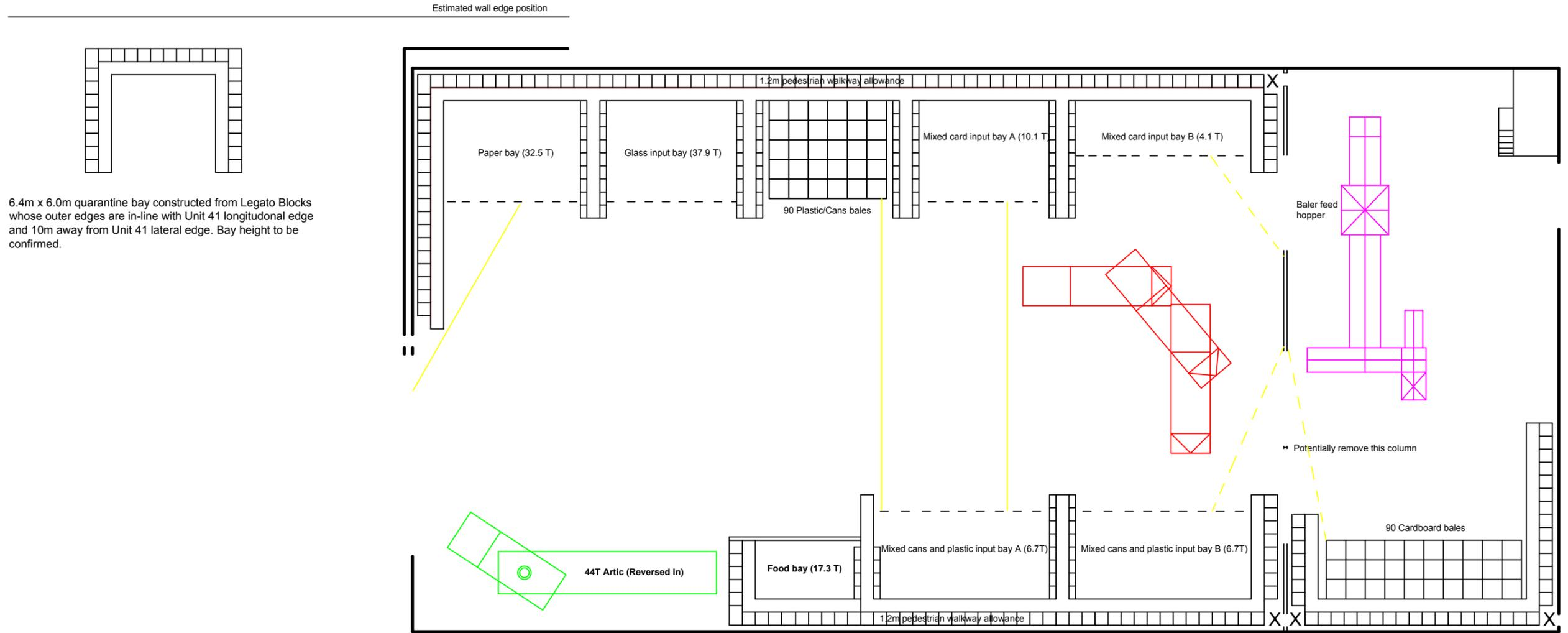
6.4m x 6.0m quarantine bay constructed from Legato Blocks whose outer edges are in-line with Unit 41 longitudinal edge and 10m away from Unit 41 lateral edge. Bay height to be confirmed.
