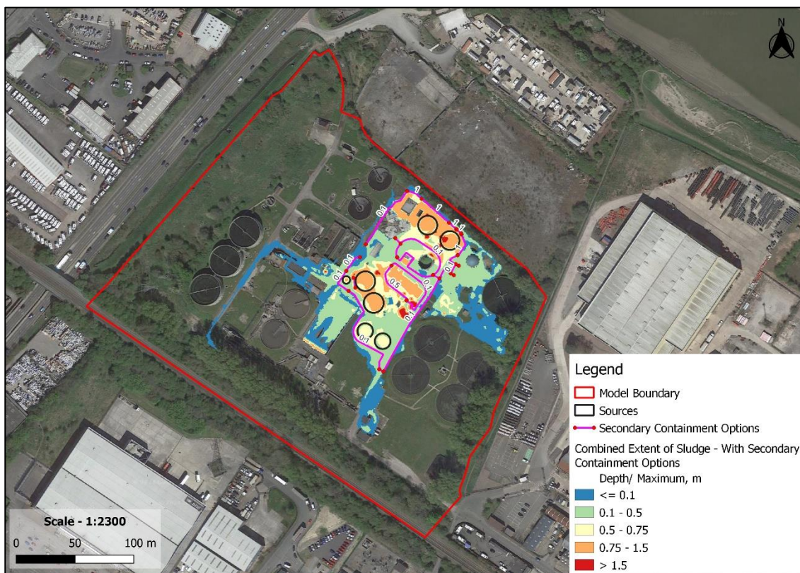
Figure 5.1: Combined Extent of Sludge from the post-failure of all sources - With Existing Secondary Containment Option
