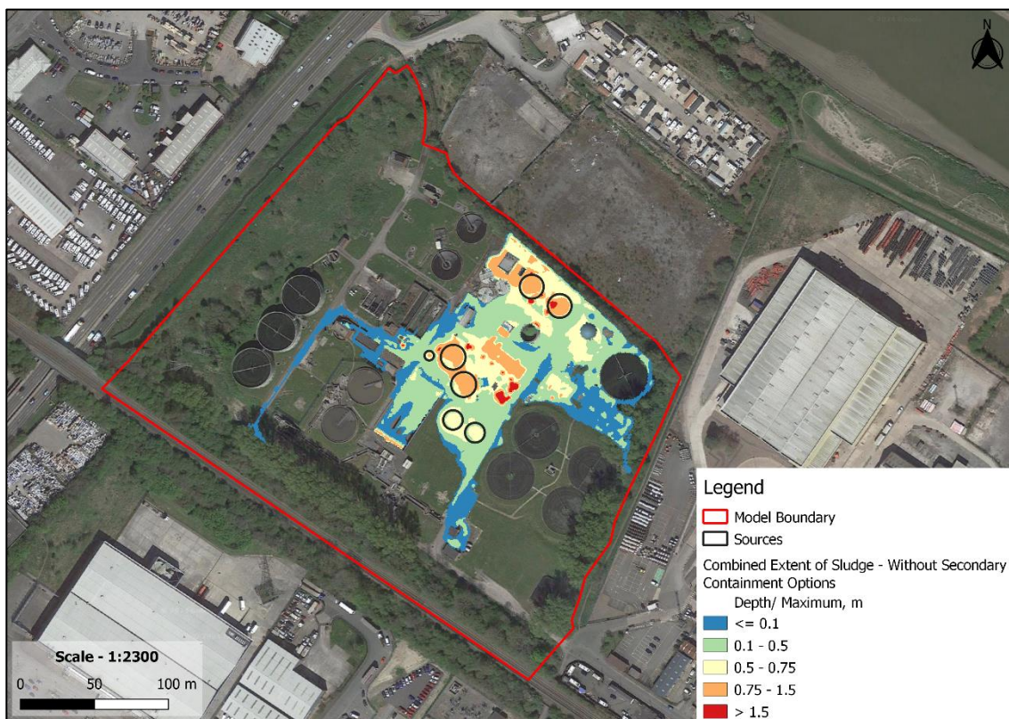
Figure 4.3: Combined Extent of Sludge from the post-failure of all sources – without Existing Secondary Containment
