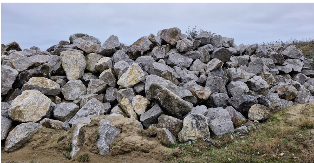
Image 9. Example of facing stone to be used along seaward edge of boundary (fence line)
