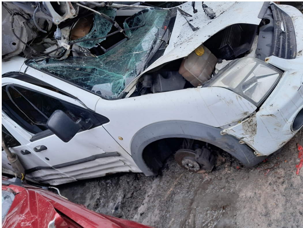
Depolluted ELV - liquid still present in the cooling system.
