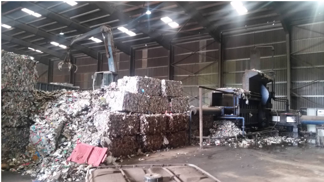
Picture 2: Steel can bales and henschel hydraulic baler.
