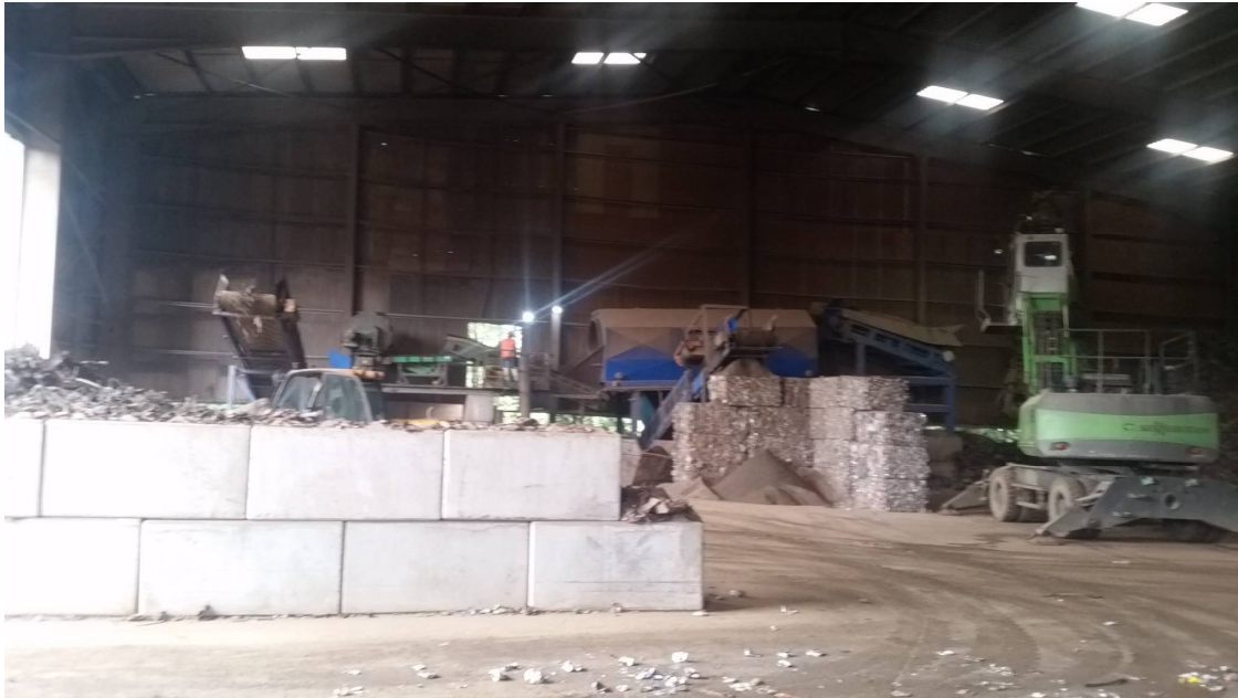
Picture 2: Kenny and Co fixed trommel and materials handler inside the factory.
