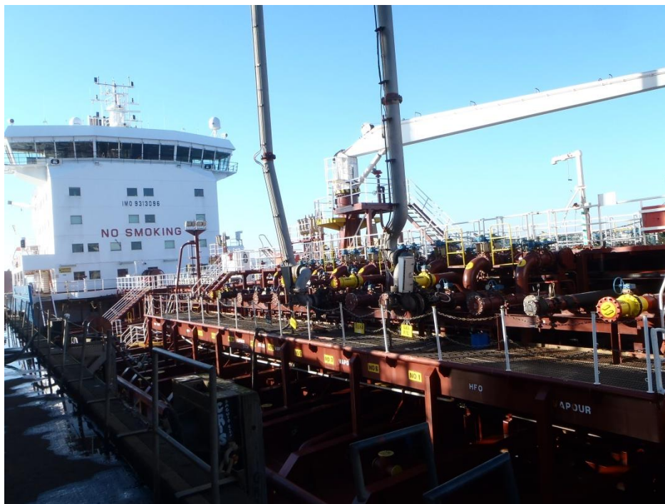
Fig 1: Typical Ship Loading via two arms. Yellow painted ship vapour connections shown.
