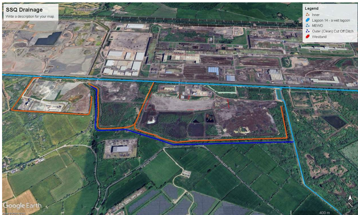
Figure 2-4 Drainage network surrounding SSQ (orange – inner dirty ditch, dark blue – outer clean ditch, light blue – MEWD that drains to pumping station)
