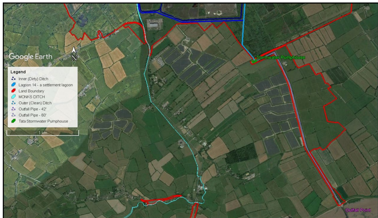
Figure 2-5 Surface water drainage system showing the Stormwater Pumphouse and Outfall Pipeline
