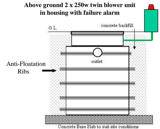
\*\* Access cover options are available for installation in vehicular / trafficked areas but CLENVIRO **MUST** be consulted at quotation stage as an alternative manufacturing structural design is required.
