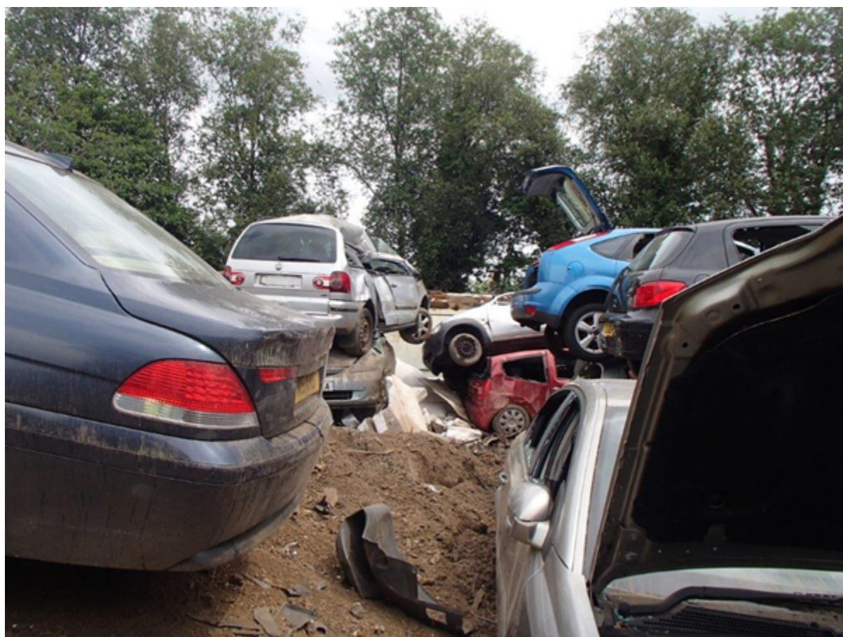
photo 2 non-depolluted vehicles stored on permeable ground
