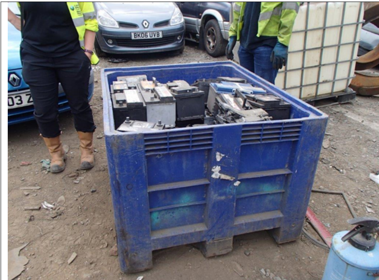
photo 9 batteries stored outside in a container with no lid and on permeable ground
