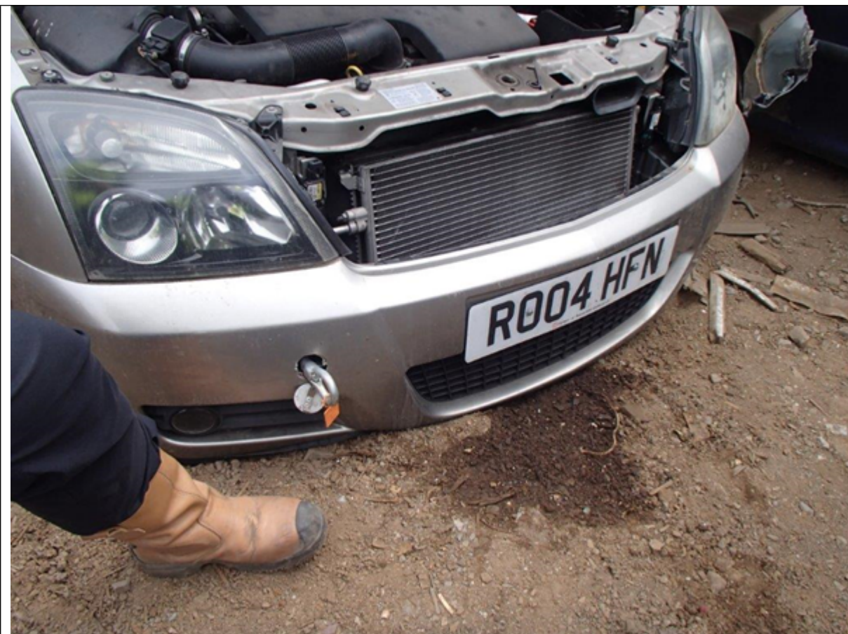
photo 1 ELV which has leaked onto permeable ground
