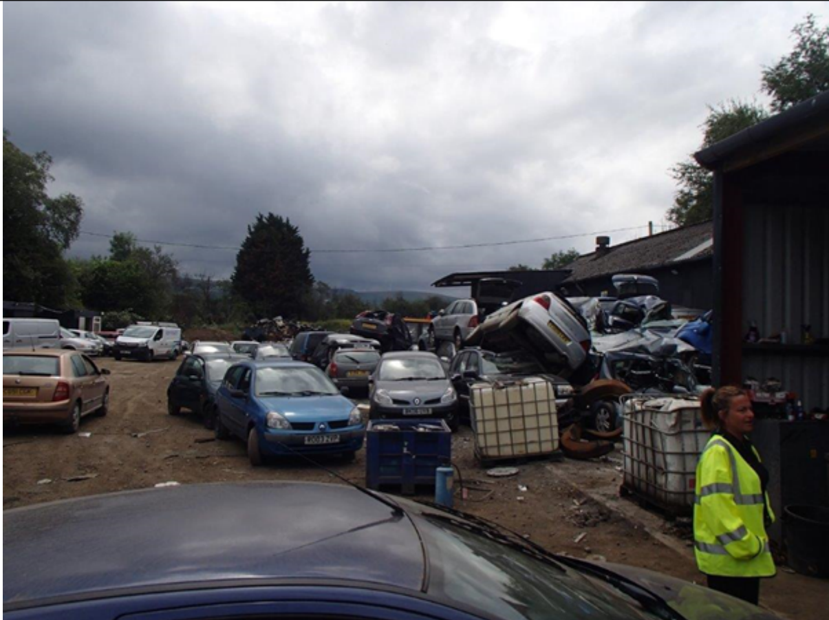
photo 3 non depolluted vehicles stored on permeable ground
