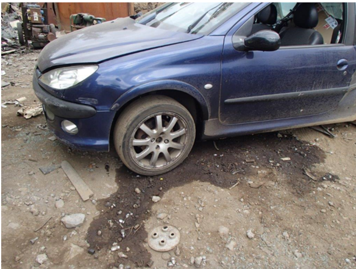
photo 4 ELV which has leaked onto permeable ground
