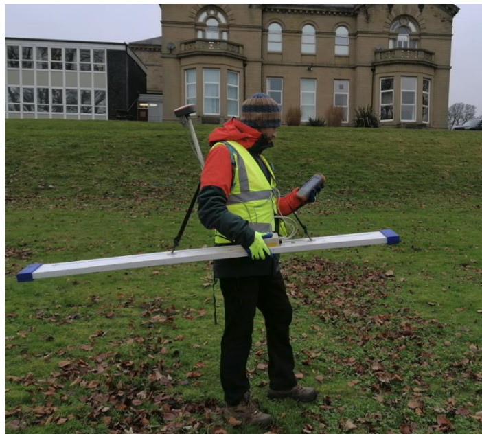
Photo 2 – Geophex GEM-2 Instrument
