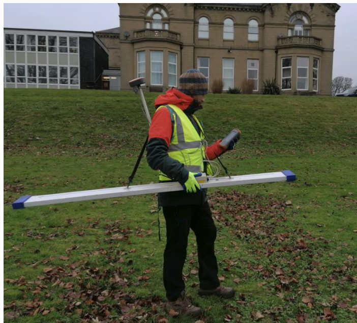
Photo 2 – Geophex GEM-2 Instrument
