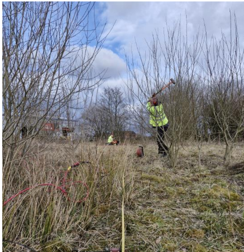
Photo 2 - ABEM Terraloc Equipment setup.
