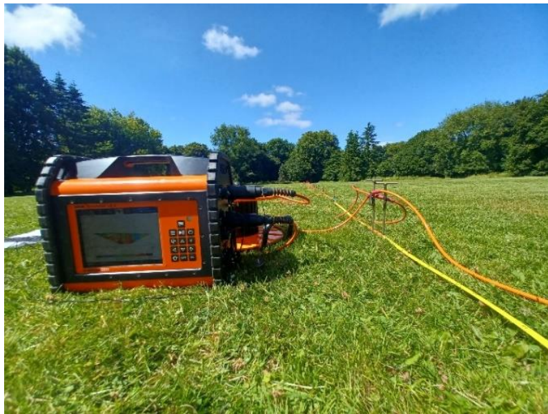
Photo 2 - ABEM LS-2 ERT Equipment setup.
