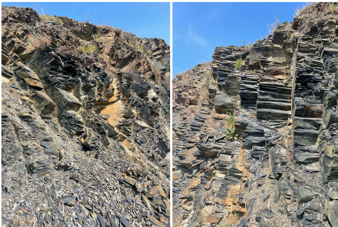
Plate 3-1 Selected exposures of bedrock on site (note widespread orange ochre staining on discontinuities compared to rock mass)
