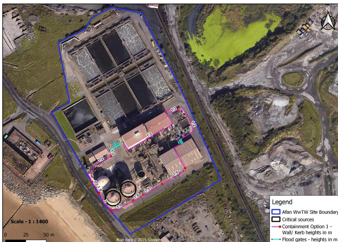
Figure 21: Proposed Enhanced Secondary Containment option
