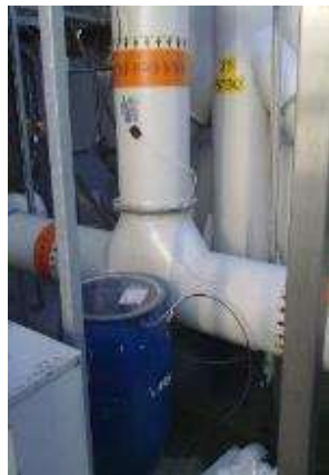
Figure 1 Point source odour sampling
