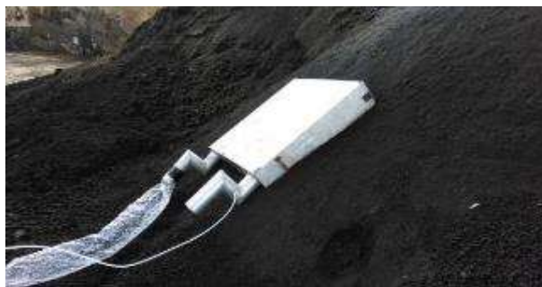
Figure 2 Picture of a Lindvall hood on a solid surface
