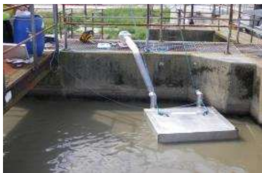
Figure 1 Picture of a Lindvall hood on a liquid surface
