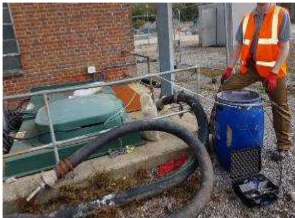
Figure 2 headspace sampling
