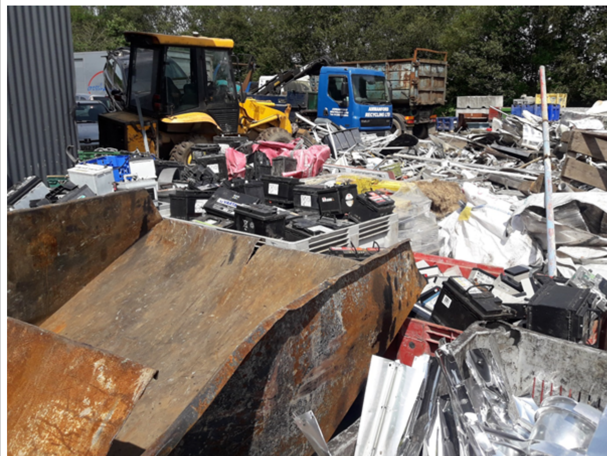
Photo 4 Batteries being stored outside in a container without a lid. This container should have been moved into the building or provide with a lid to prevent the ingress of water. This action was not carried out.
