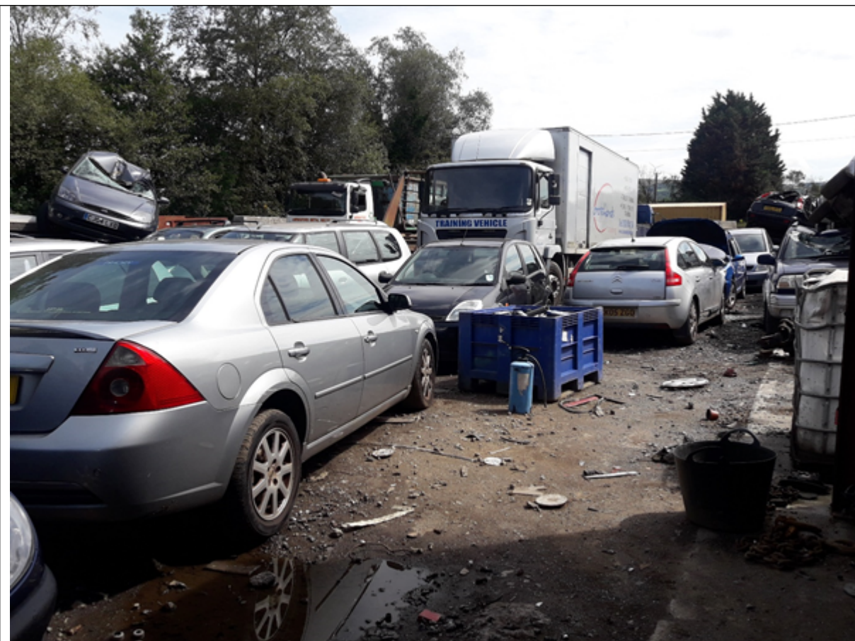
Photo 4 Batteries being stored outside in a container without a lid. This container should have been moved into the building or provide with a lid to prevent the ingress of water. This action was not carried out.
