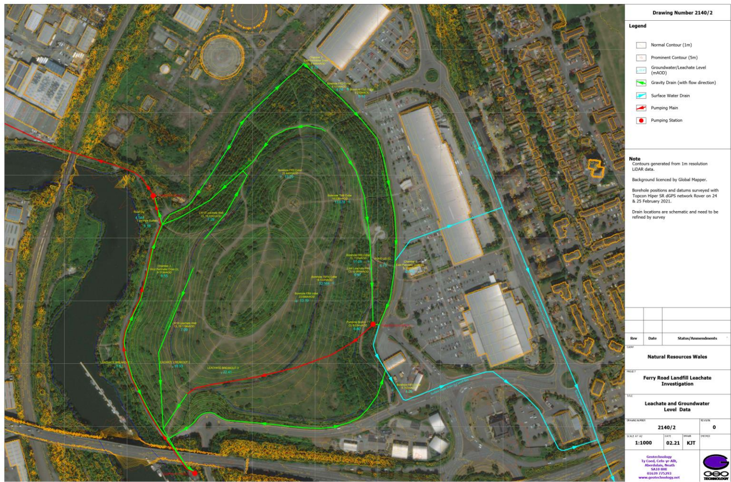
Figure 3.8: Plan showing leachate drainage
