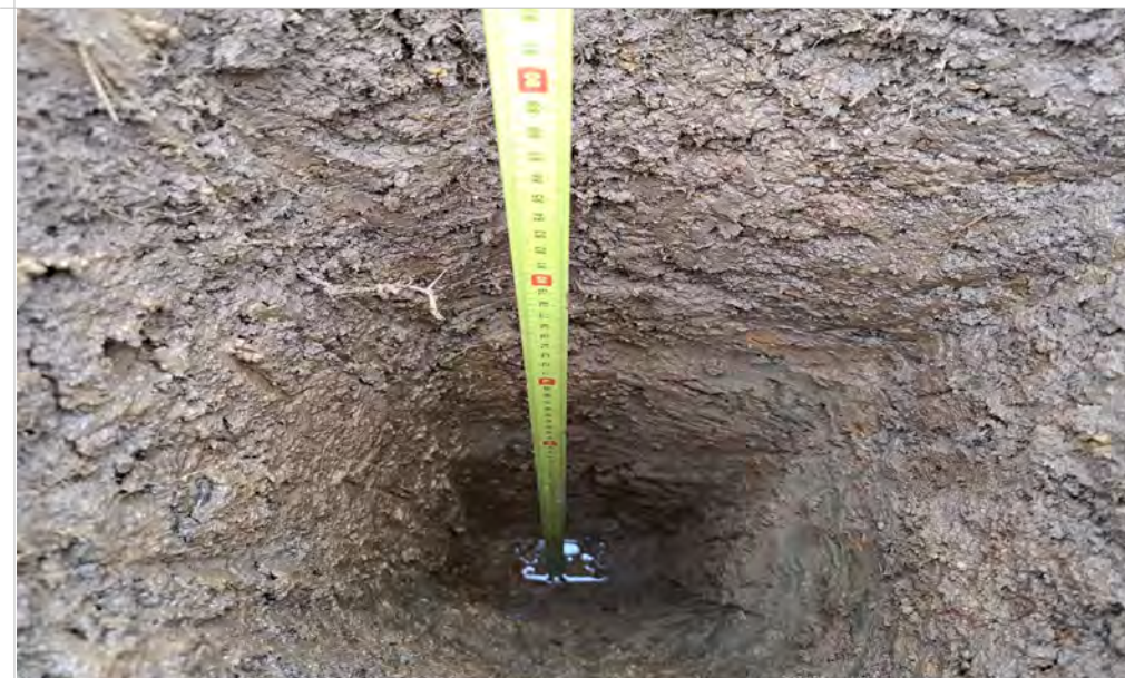
Plate 19: WS09 Hand Pit 0.00m to 1.20m bgl.
