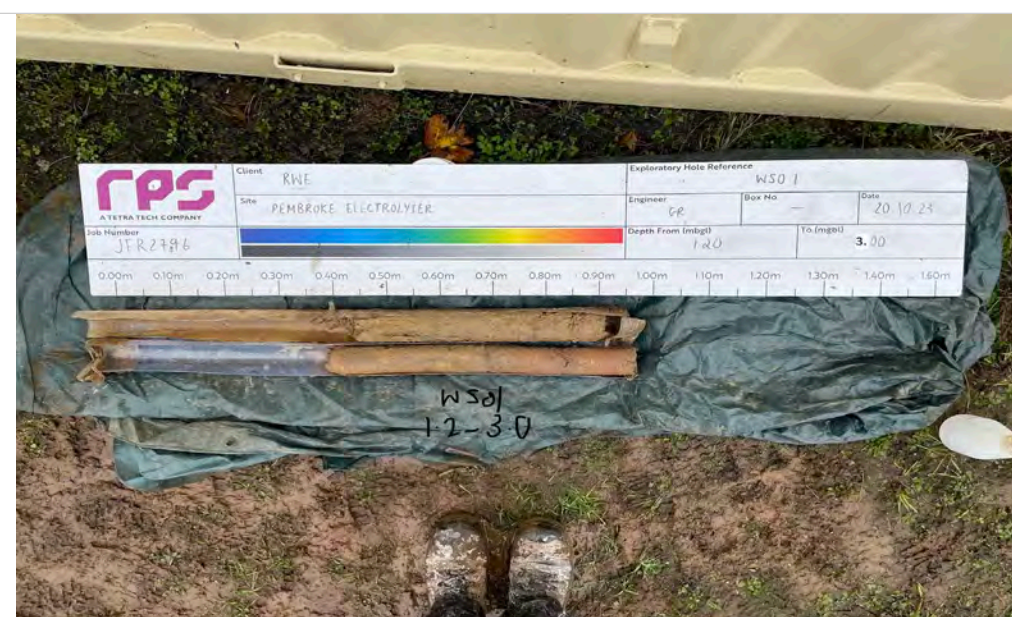
Plate 02: WS01 Sample Recovery 1.20m to 3.00m bgl.
