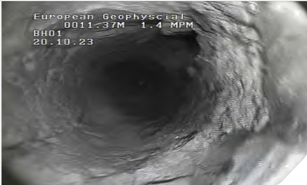
Plate 11: BH01 downhole view at 11.37 m bgl. Collapsed material associated with near vertical jointing.
