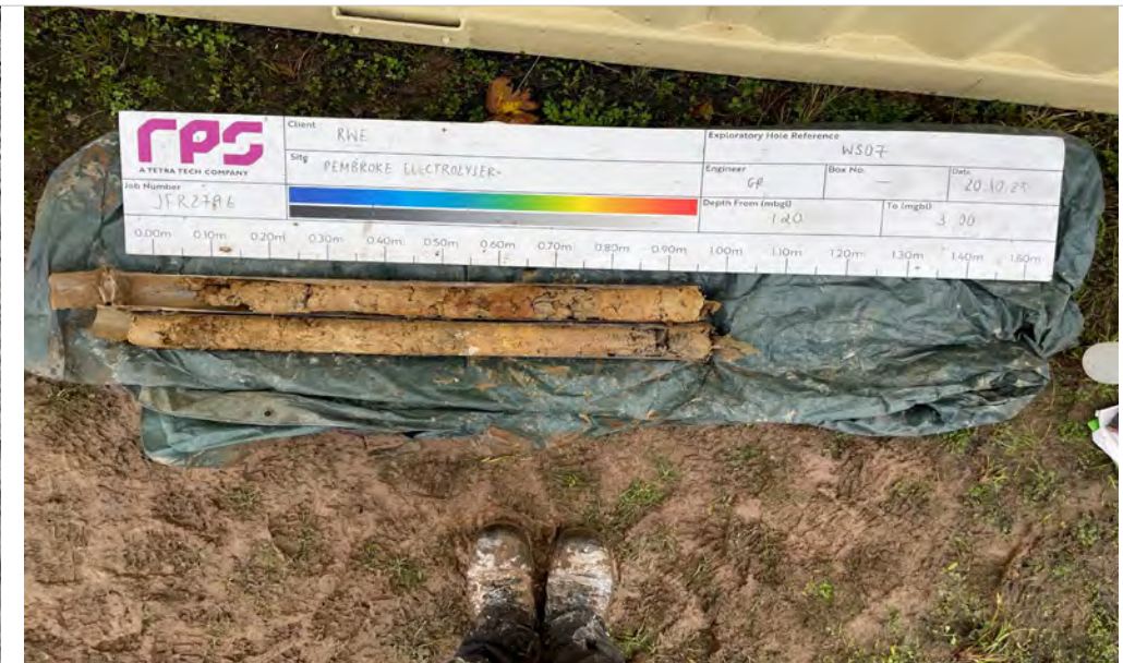
Plate 16: WS07 Sample Recovery 1.20m to 3.00m bgl.
