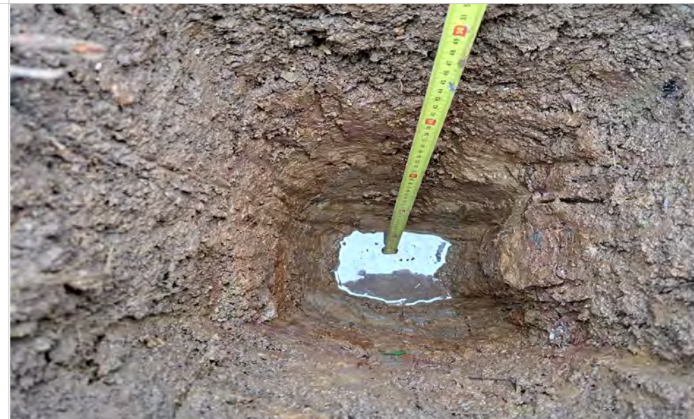
Plate 15: WS07 Hand Pit 0.00m to 1.20m bgl.
