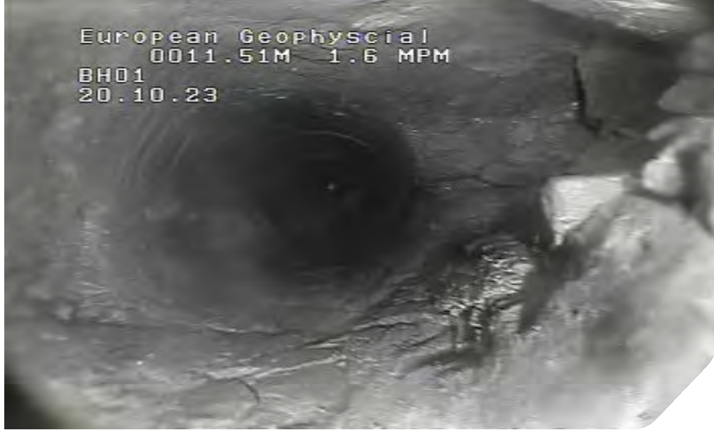
Plate 10: BH01 downhole view at 11.51 m bgl. Collapsed material associated with near vertical jointing.
