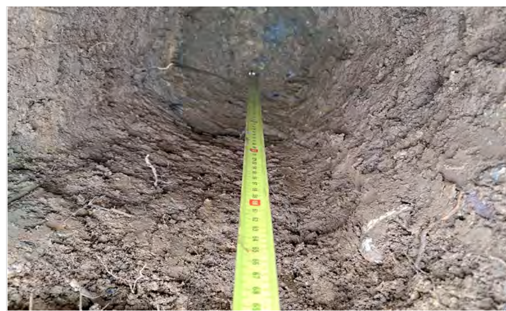
Plate 13: WS06 Hand Pit 0.00m to 1.20m bgl.
