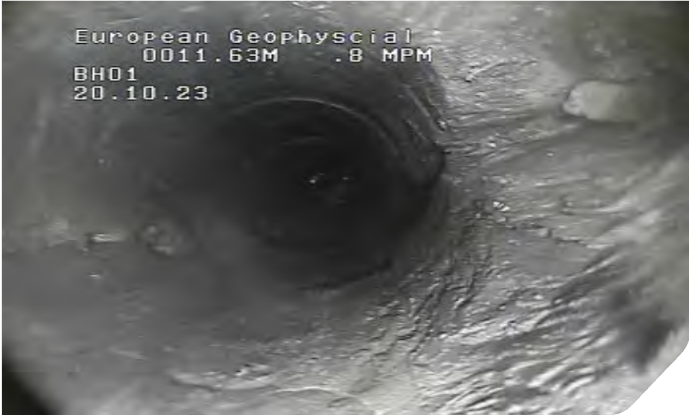
Plate 09: BH01 downhole view at 11.63 m bgl. Collapsed material associated with near vertical jointing.
