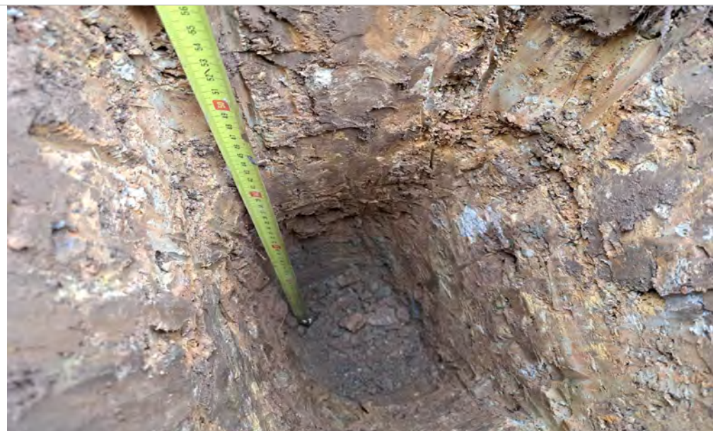
Plate 08: WS04 Hand Pit 0.00m to 1.20m bgl.
