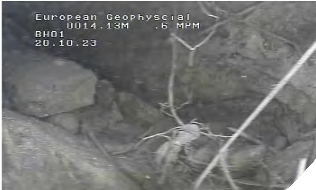
Plate 03: BH01 downhole view at 14.13 m bgl. Open void, no borehole walls visible.
