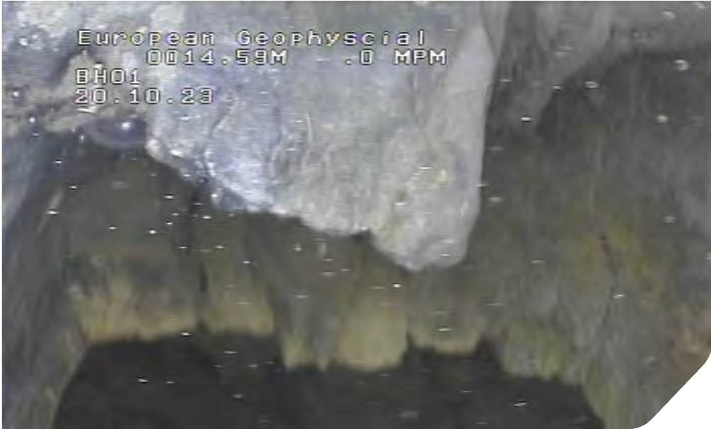
Plate 01: BH01 side view at 14.59 m bgl. Natural void, dimension and orientation unknown.
