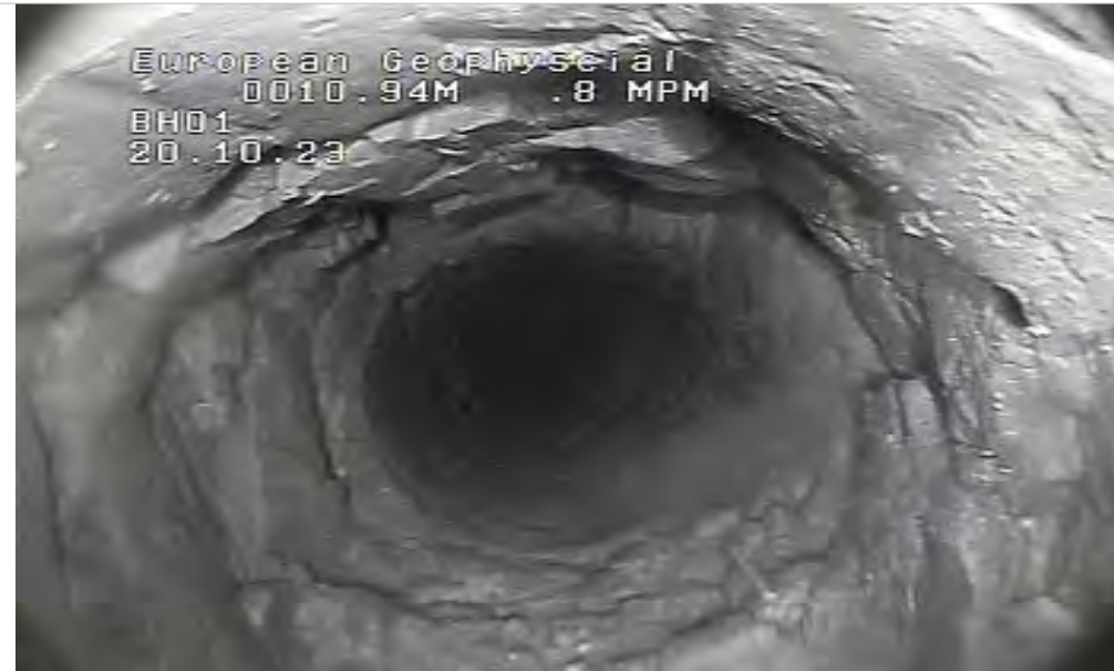
Plate 12: BH01 downhole view at 10.94 m bgl. Loose borehole sidewall, collapsed material due to jointing.
