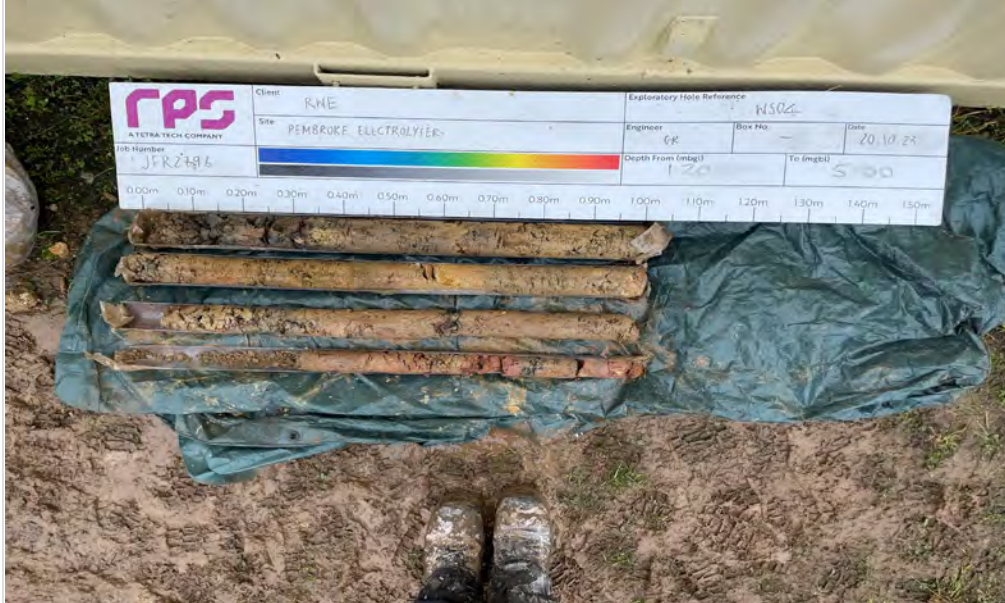
Plate 09: WS04 Sample Recovery 1.20m to 5.00m bgl.
