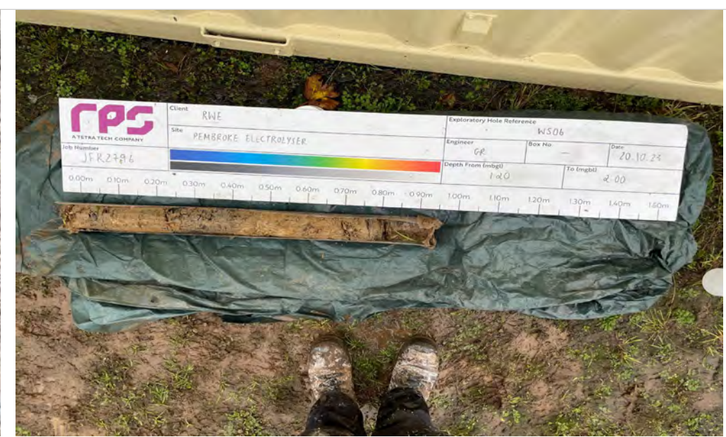
Plate 14: WS06 Sample Recovery 1.20m to 2.00m bgl.
