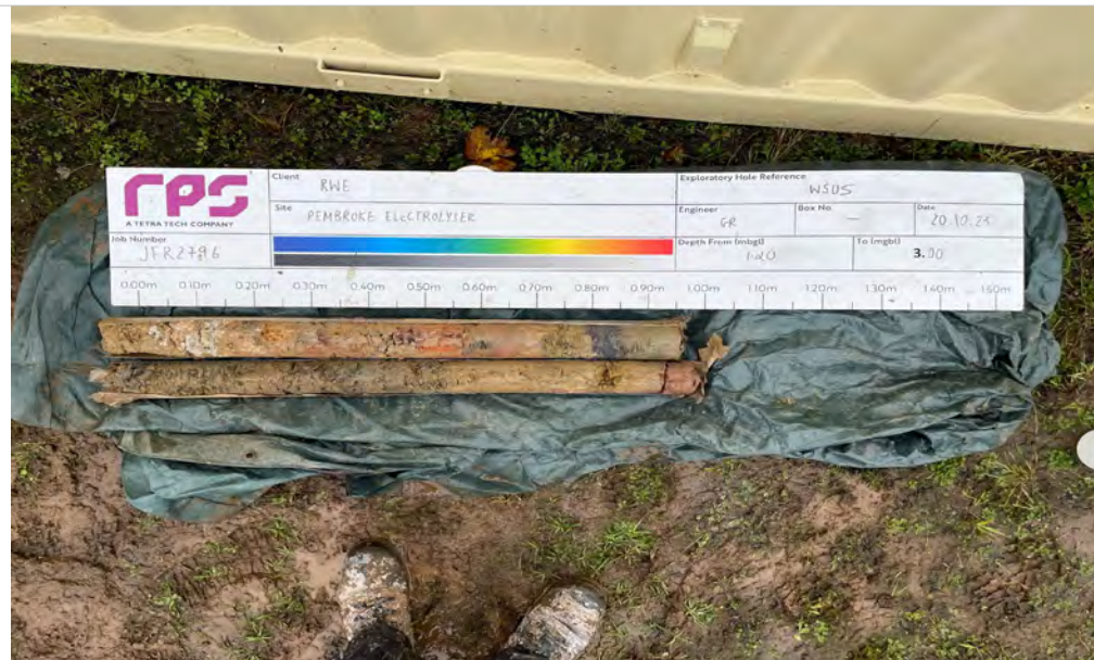
Plate 12: WS05: Sample Recovery 1.20m to 3.00m bgl.
