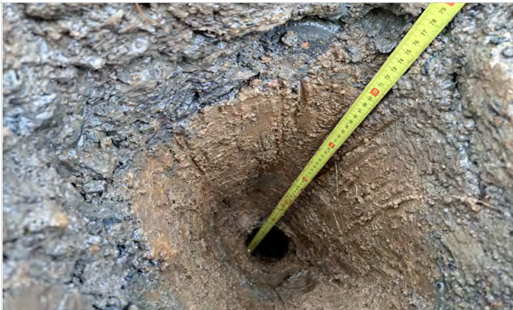
Plate 11: WS05 Hand Pit 0.00m to 1.20m bgl.
