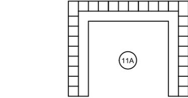
6.4m x 6.0m quarantine bay constructed from Legato Blocks whose outer edges are in-line with Unit 41 longitudinal edge and 10m away from Unit 41 lateral edge. Bay height to be confirmed.
