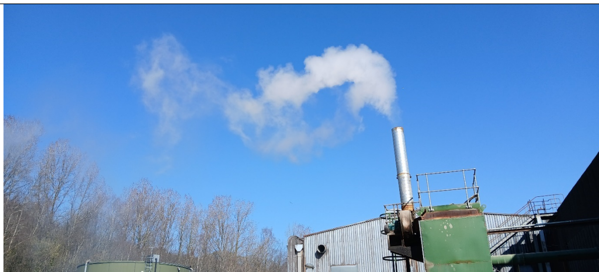
Photo 2 – Showing the moisture coming from the dryer after changing over to gas.
