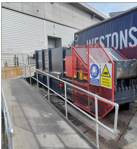
Image 2 – showing the PortaPacker unit fitted with a solid connector pipe at the base
