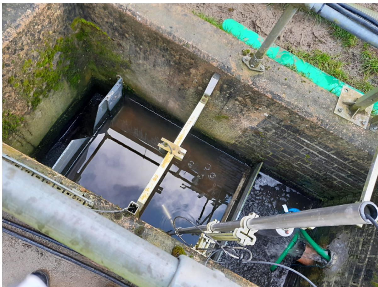
Figure 1. Photograph of V notch discharge gauge.
