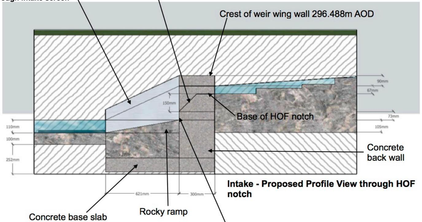
73mm - fall from the base of the slope of the HOF notch to the base of the rock ramp easement (below the HOF notch)
