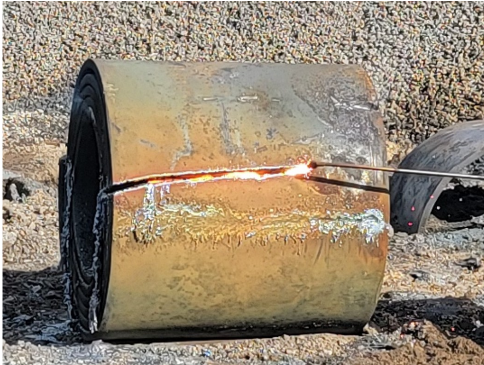
Figure 4: Oxy-propane cutting in progress (at previous processing location)
