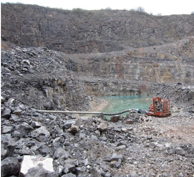
Plate 3: Sump pump in quarry void
