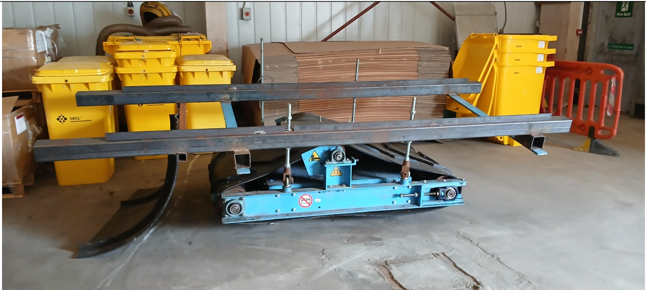
Photo 2 - Removed magnet separator which would sit on exit of line following treatment of waste(s)
