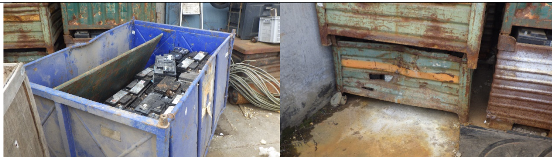
Batteries stored in an open top container and in a perforated container under cover
