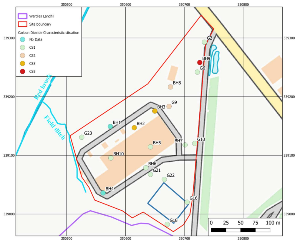
Figure 8.2: Worst case characteristic situation for carbon dioxide
