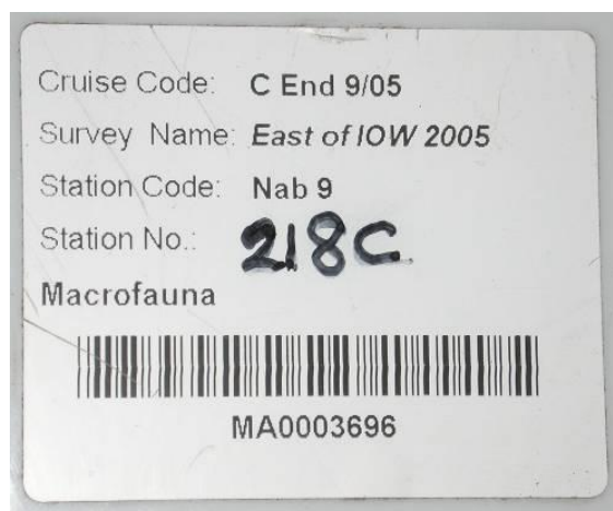
Fig. 14. Example of a pro-forma, bar-coded, printed label for a macrofaunal sample. The field for 'Station Number' is completed manually; here showing Station 218, Replicate C. All other fields are printed on the label.
