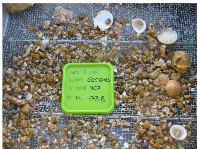
Fig. 13. Photograph of material from the sample retained on the 5mm coarse mesh sieve that sits inside the sieving table, including meta-data label (Tupperware lid).
