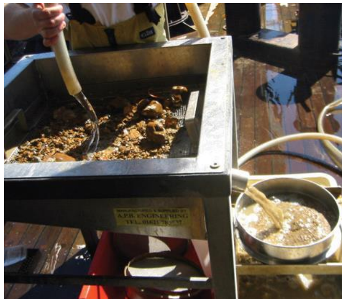
Fig. 11. Sample processing using a purpose-built sieving table. The sample is being washed over a 5 mm square mesh aperture sieve supported by a removable square stainless-steel frame. Note also the 1 mm mesh sieve held within a sieve holder beneath the outlet pipe of the table.
