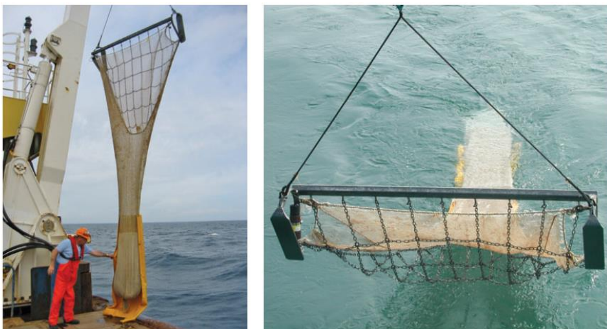
Fig. 18. 'Jennings' 2 m Beam Trawl with metal beam (Cefas © Crown Copyright 2011).
