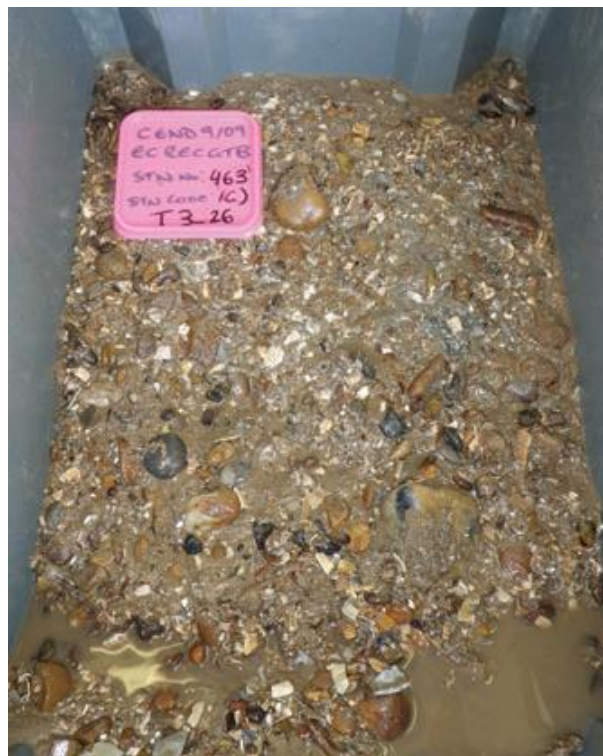
Figure 10. Photograph of Hamon grab sample, including meta-data label (Tupperware lid) taken prior to processing.
