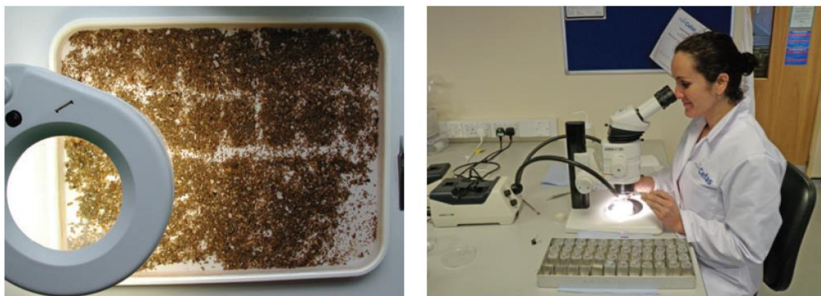
Fig. 23. (left) Gridded tray containing sorted sample. Note the illuminated magnifier. (right) Binocular microscope being used for specimen identification (Cefas © Crown Copyright 2011).
