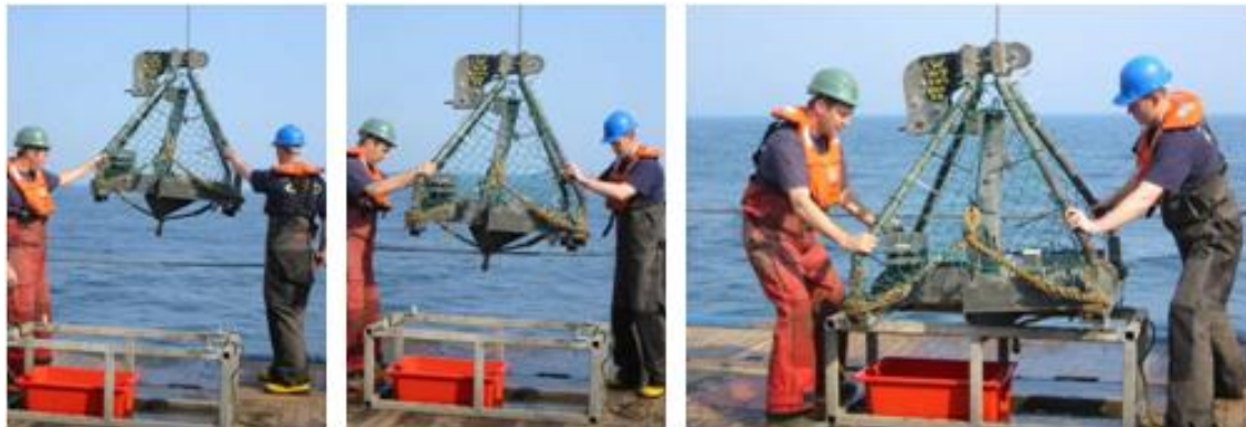
Fig. 9. Deployment and recovery of the Hamon Grab.
