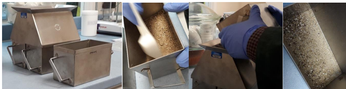
Fig. 24. 1: Sample divider; 2: Sample being mixed prior to dividing, 3: Sample added to sample divider, 4: Subsample from sample divider (Fugro) (Cefas © Crown Copyright 2020).
