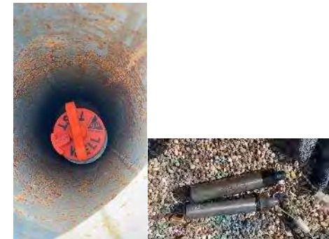
BH RC11. Upstand 0.39 m, two divers installed.
