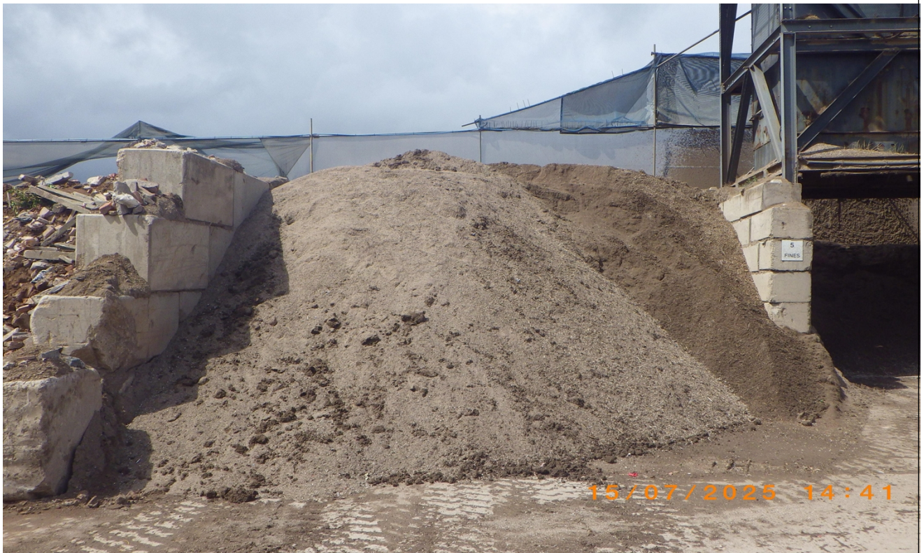
Resulting pile of fine material from BlueMAC process.
