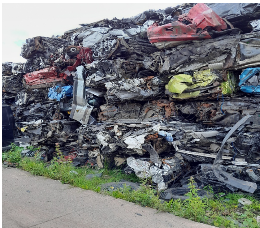
Photo 3 - Storage of scrap, baled metal exceeding 4 metres.
