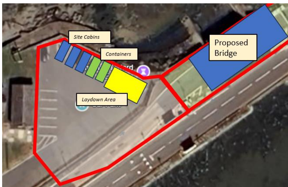
Figure 1 – Indicative Compound Arrangement (Picture source Google.com/maps)
